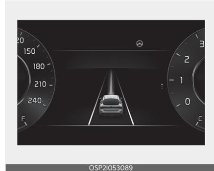
If the vehicle ahead or both lane markings are detected and your vehicle speed is below 180 km/h (110 mph), the green (🚗) indicator light will illuminate on the cluster, and the function will help centre the vehicle in the lane by controlling the steering wheel.
