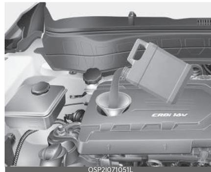
Use only the specified engine oil. (Refer to "Recommended lubricants and capacities" on page 9-10.)
