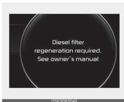
If the warning message "Diesel filter regeneration required, See owner's manual." appears on the LCD display, Self Regeneration is required.
