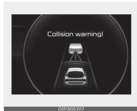
Whilst Smart Cruise Control is operating, when the collision risk with the vehicle ahead is high, the warning message will appear on the cluster, and an audible warning will sound to warn the driver. Always have your eyes on the road whilst driving, and if necessary, depress the brake pedal to reduce your driving speed in order to maintain a safe distance.
