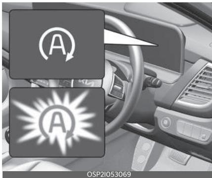
ISG system is indicated by the green AUTO STOP indicator (A) on the instrument cluster.
