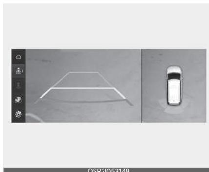
Parking distance warning is displayed on the right side of the Surround View Monitor top view screen when the **Parking distance warning** is selected.
