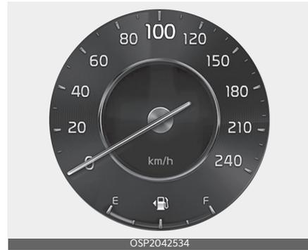
The speedometer indicates the speed of the vehicle and is calibrated in kilometers per hour (km/h).
