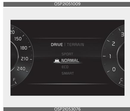
1. **NORMAL mode:** NORMAL mode provides soft driving and comfortable riding.
