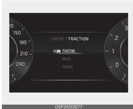
If you press the "DRIVE/TRACTION" mode button, the driving mode is changed from Driving control to Traction control. You can select SNOW (1), MUD (2) or SAND (3) mode by rotation the knob. If you press the "DRIVE/TRACTION" mode button again, the driving mode is changed from Traction Control to previous driving control.
