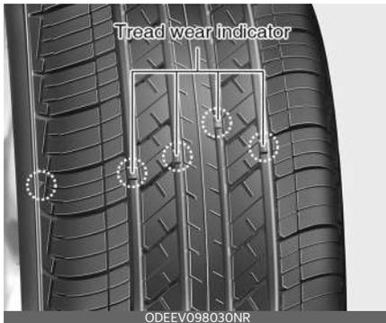
This shows there is less than 1.6 mm of tread left on the tyre. Replace the tyre when this happens.
