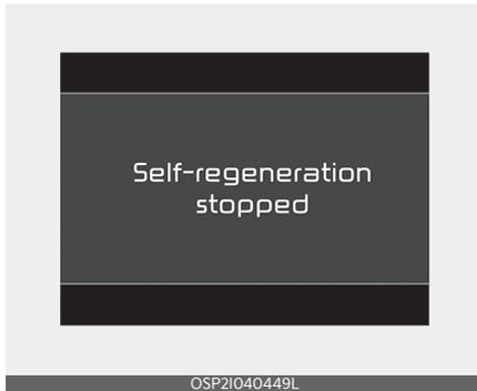
The regeneration operation could be cancelled if the driver press the OK button firmly whilst operating the self regeneration process.
