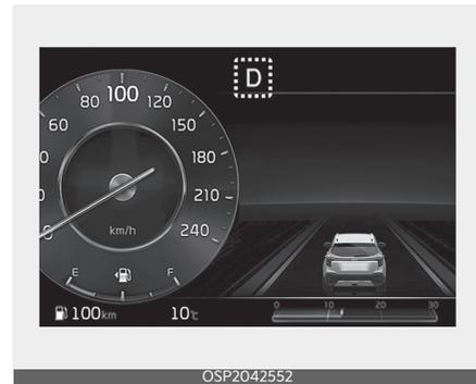
This indicator displays which automatic transmission shift lever is selected.
