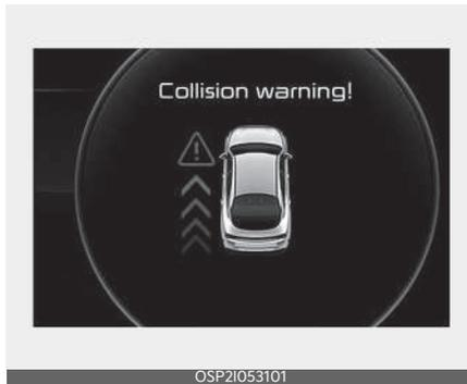
The warning light on the side view mirror will blink and the warning message will appear on the cluster, and an audible warning will sound.
