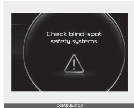
When Blind-Spot Collision-Avoidance Assist is not working properly, the warning message will appear on the cluster for several seconds, and the master (⚠) warning light will appear on the cluster for several seconds. If this occurs, have the vehicle checked by a professional workshop. Kia recommends to visit an authorized Kia dealer/service partner.
