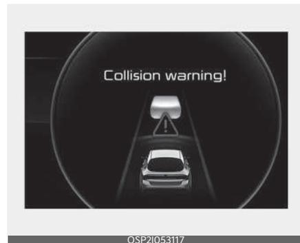
Collision warning will alert the driver with a warning message, an audible warning and steering wheel vibration (if equipped).
