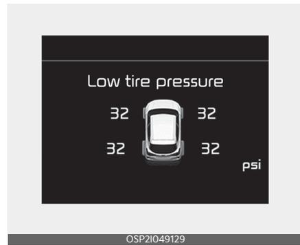
The low tyre pressure position telltale light will indicate which tyre is significantly under-inflated by illuminating the corresponding position light.
