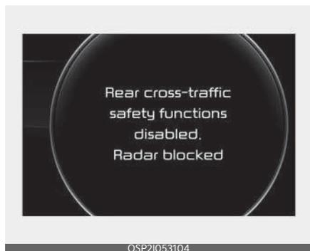
When the rear bumper around the rear-side radar or sensor is covered with foreign matters, such as snow or rain, or installing a trailer or carrier, it can reduce the detecting performance and temporarily limit or disable Safe Exit Warning.
