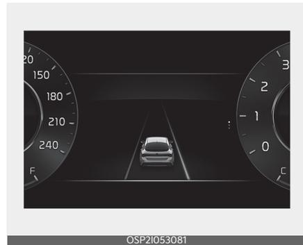
Lane Keeping Assist will warn and help control the vehicle with Lane Departure Warning and Lane Keeping Assist.
