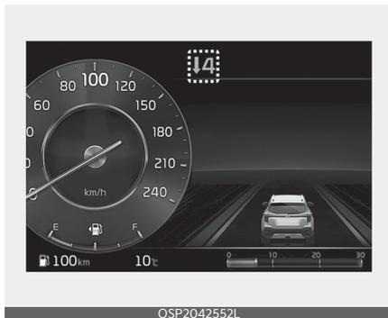
This indicator informs which gear is desired whilst driving to save fuel.
