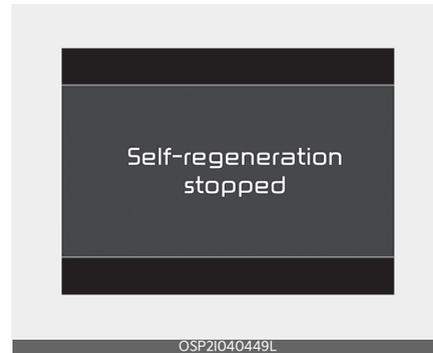
The self regeneration process stops if any of the self regeneration conditions is cancelled. If the self regeneration process is cancelled automatically, the system maintains "Self-regeneration stopped" message. If the driver press the OK button firmly, it can restart the self regeneration mode again. (Self regeneration conditions should be satisfied.)
