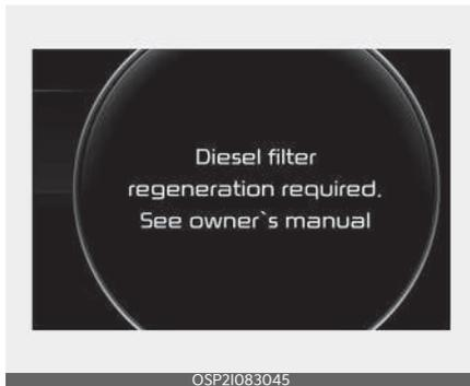
If the system still needs the self regeneration process after cancelling the operation, the warning message appears. (Diesel filter regeneration required.) If the driver press the OK button firmly, it can restart the self regeneration mode again. (The Self regeneration conditions should be satisfied.)
