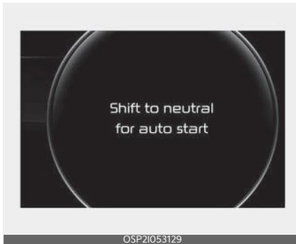
**Automatic Transmission** - Place the transmission shift lever in P (Park). Depress the brake pedal fully. You can also start the engine when the shift lever is in the N (Neutral) position.
