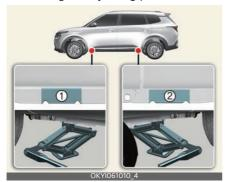
Insert the jack handle into the jack and turn it clockwise. Raise the vehicle until the tyre just clears the ground. Make sure the vehicle is stable before removing the wheel lug nuts.
