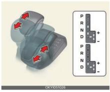
Depress the brake pedal and the lock release button when shifting.
