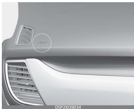
Passenger's front air bag
